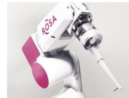
ROSA has two main parts: a computer "brain" for 3-D imaging and stereotactic planning, and a robotic arm that directs surgical instruments with extreme accuracy. For epilepsy surgery, ROSA helps the surgeon to place a series of very fine electrodes deep within the brain to detect where seizures are coming from. The electrodes are placed in a safe, exact and minimally invasive fashion, which not only improves the precision of the procedure, but speeds the recovery.
